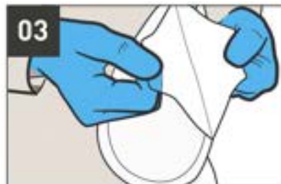
03 PEEL OFF the protective liner, exposing the adhesive portion of the seal
